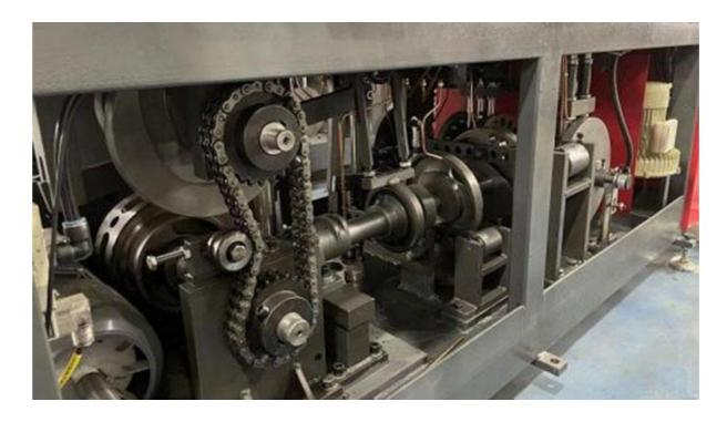
1. The whole **Middle Speed Paper Cup Machine** adopts automatic oil lubrication system( oil circulation system is including oil motor, filter, copper pipe) which makes all gear moving parts working at high speed much more smoothly and greatly Improve the service life of spare parts.
